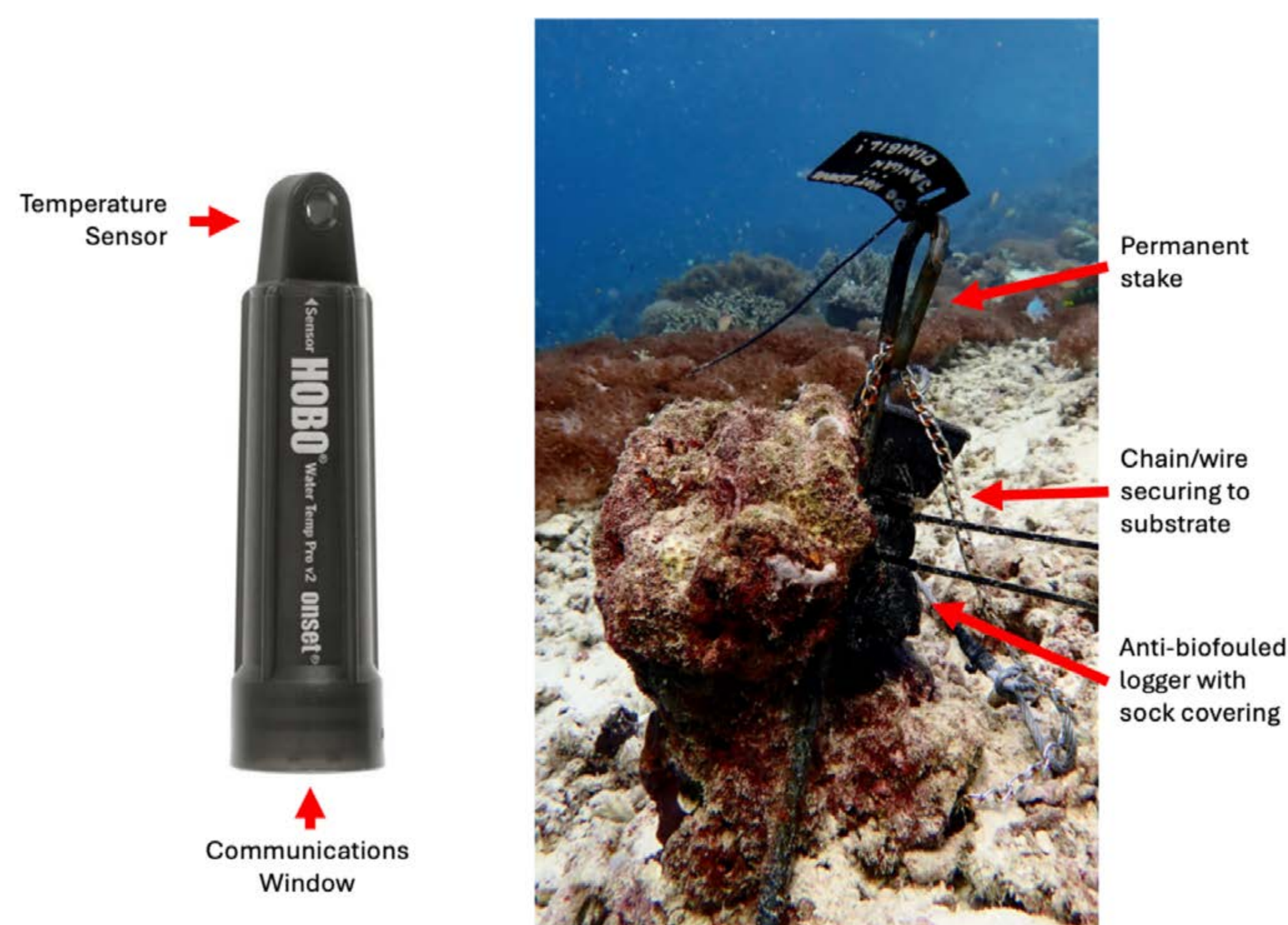
Image 1 Diagram depicting a HOBOWare V2 Temperature Logger used to collect data. Different aspects of the logger are indicated as well as an image of a deployed logger off Barefoot Jetty, complete with anti-biofouling gear and other equipment (ie. stake) to permanently secure to the substrate.
